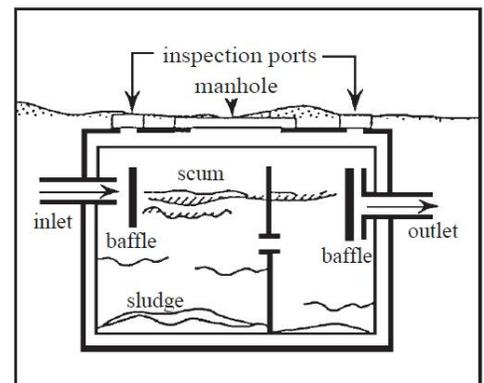
Figure 2: **A Two-Compartment Septic Tank**—Courtesy National Small Flows Clearinghouse
