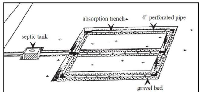
Figure 1: **Septic System**—Courtesy National Small Flows Clearinghouse
