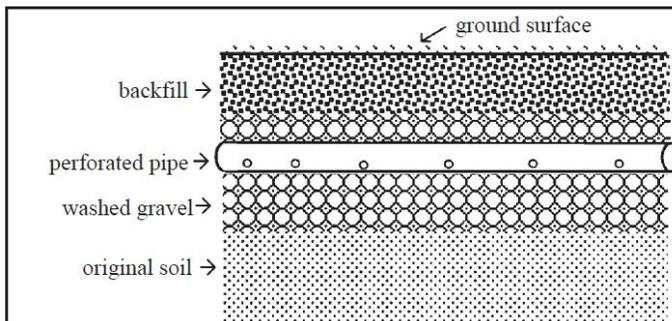
Figure 4 Septic Drainfield, Courtesy—Washington State University
